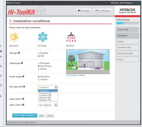
Each heat pump system has a water tank, some of which are optional, depending on the solution found. When a water tank is selected, an extra tab appears to fill in the water tank selection.
