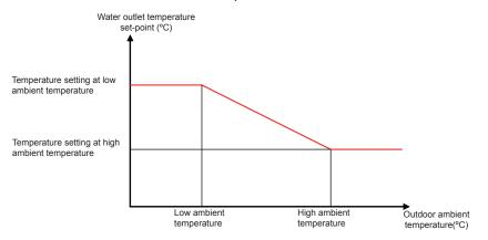
• OTC Gradient (Only for heating space): Water target is selected by an Outside Temperature Compensated (OTC) control that is defined by a different gradient of the curve. The initial point of the curve is always 20°C-20°C (Water outlet target 20°C at outdoor ambient temperature of 20°C).
