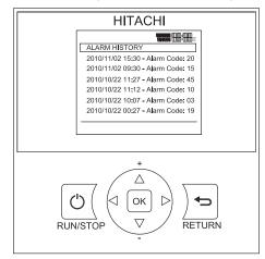
The software can save up to the last 20 alarms, showing on the screen the following data:
