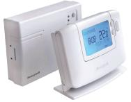
Intelligent room thermostat unit (accessory) with extension room thermostat (accessory) for the second circuit: Based on Outside Temperature Compensation (OTC). Water outlet target temperature is automatically recalculated taking into account the outdoor ambient temperature and the difference between the room setting temperature and the room actual temperature.
