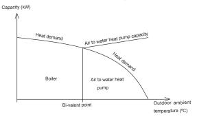
Boiler for emergency mode (Optional function): In case of outdoor unit malfunction, the heating required can be provided by the boiler.
