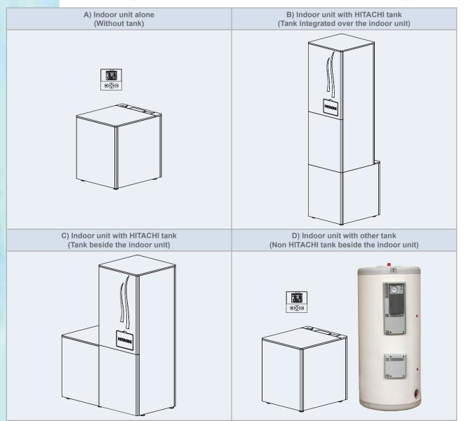
Depending on the configuration type, the installation procedure will be different.
