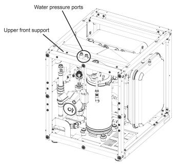
Plug in a differential manometer to the pressure ports and open the inlet / outlet ports (1\*).
