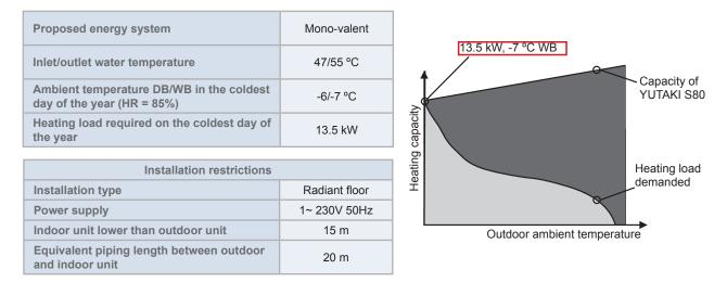
These conditions will determine the entry in the maximum heating capacity tables (see section *Maximum heating capacity tables*) where it is possible to identify which unit has the heating capacity to cover the required heating load on the coldest day of the year by the installation (13.5 kW for an inlet/outlet water temperature of 47/55 °C and an ambient temperature of -7°C WB).
