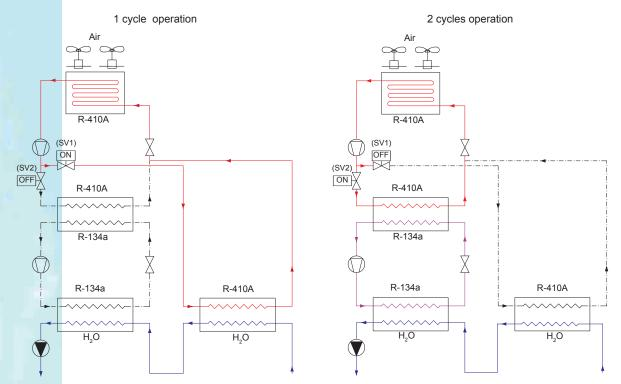
The innovative SMART cascade cycle results in a better COP than cascade conventional cycles, because it leverages the best working conditions for any moment.
