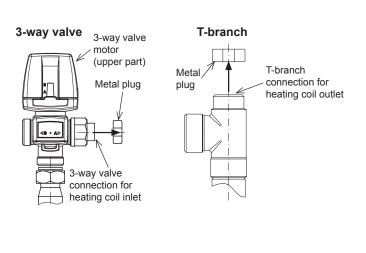
3-way valve connection T-branch connection for for heating coil inlet heating coil outlet
