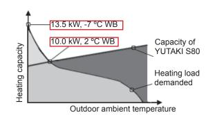
In this new system the heat pump meets with the regular heating load. To reach the peak heating load of 13.5 kW (-7°C WB) necessary in the coldest days of the year the electric heater can provide the auxiliary heating capacity to cover it.
